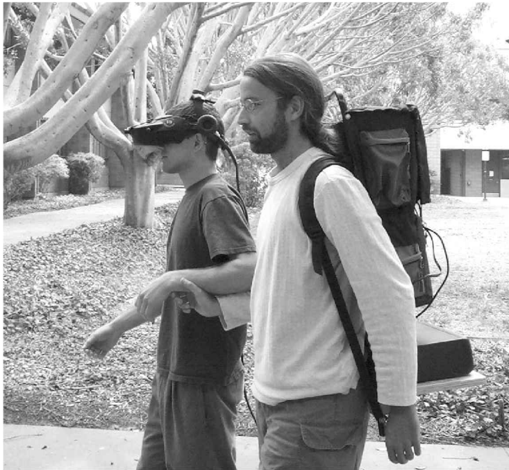
Figure 2. Photograph of the experimenter and participant in the walk condition during learning. The experimenter's backpack contained video recording equipment and a power supply. It was connected to a head-mounted display worn by the participant. A small camera, mounted to the front of the display, provided on-line visual information to the participant.
