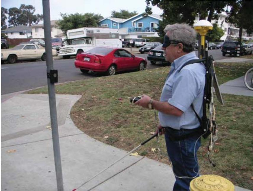
Fig. 4. First author using the HPI RIAS interface to locate an infrared transmitter at a bus stop, street waypoint 4.
