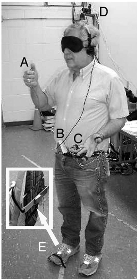
Figure 1. Apparatus for the navigation task: (A) push button, (B) body orientation sensor, (C) vibrator on finger, (D) head orientation sensor, (E) footstep sensor (also shown in inset).
